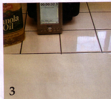
3 Oil penetrates to back side.
